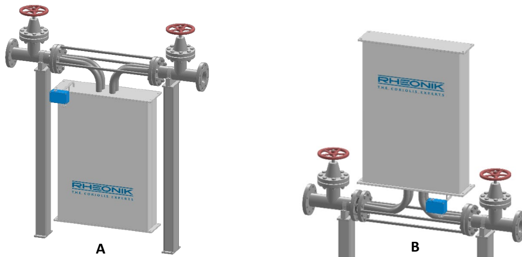
Figure 7: Installation positions for liquid (A) and liquid applications with solid particles/gas applications (B)
